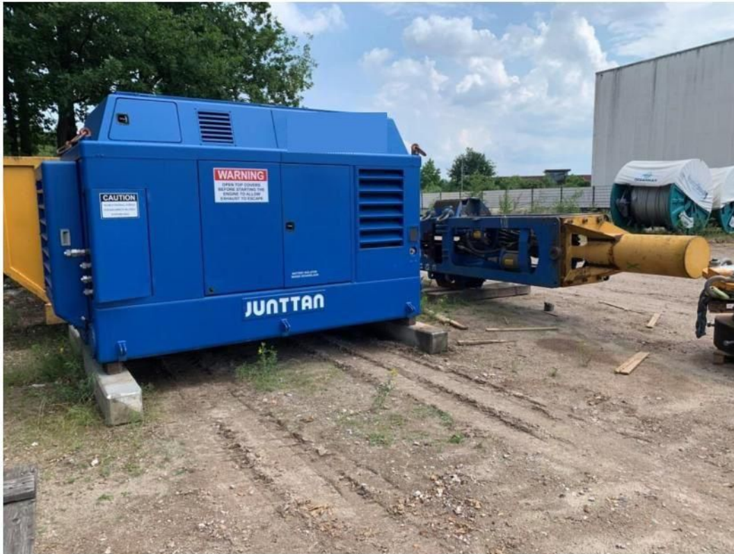
Original Junttan 15CCU power pack with Cummins engine, tier III, biodegradable oil
